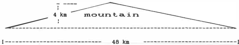
Fig. 2. Comparison of Stokes formulae (the classical method), and the method of Molodensky, for determination of the deviation of the vertical under a mountain of height 4 km
