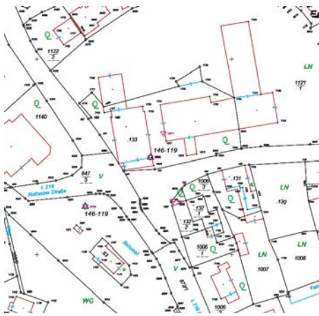
Figure 4: Example of a digital cadastral map (DKM) used for fixing the horizontal position of the gravity stations.
