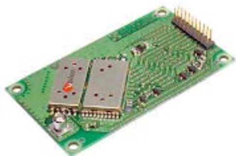
Figure 3: EMAG functional demonstrator overview (left: u-blox GPS/EGNOS receiver module; right: NAUTICAST AIS transponder).
