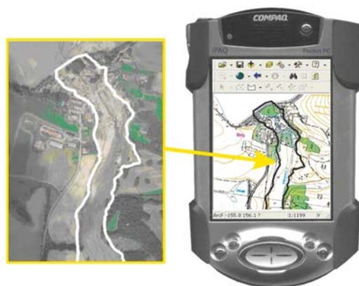
Fig. 5: Data capture and updating of objects in flood area Fig. 6: Survey extent of flooding line
