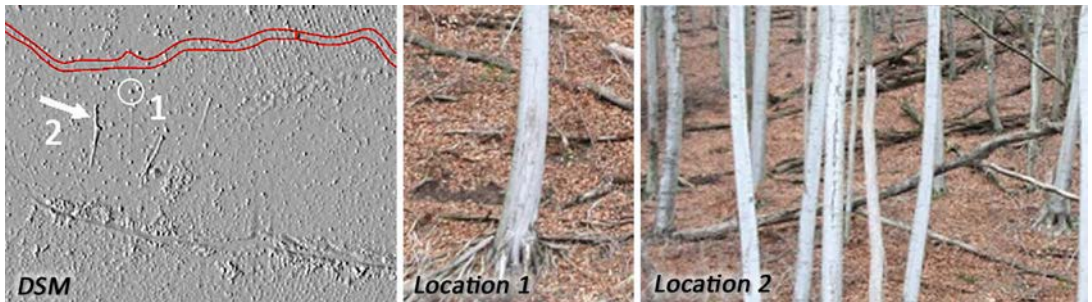
Fig. 4: DSM produced from full-waveform ALS point cloud cut of at 2 m height difference to DTM. Individual and fallen trees are clearly visible. The two images on the right were taken on-site and geo-referenced with GPS. [55]
