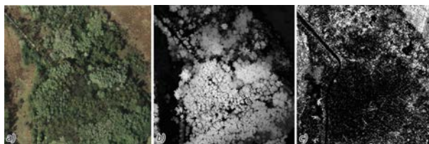
Fig. 5: (a) Orthophoto; (b) nCM (white = high); (c) ratio of points below 0.2 m and in between 0.2 and 2 m (black = only points below 0.2 m), linear structures correspond to fallen trees. [68]
