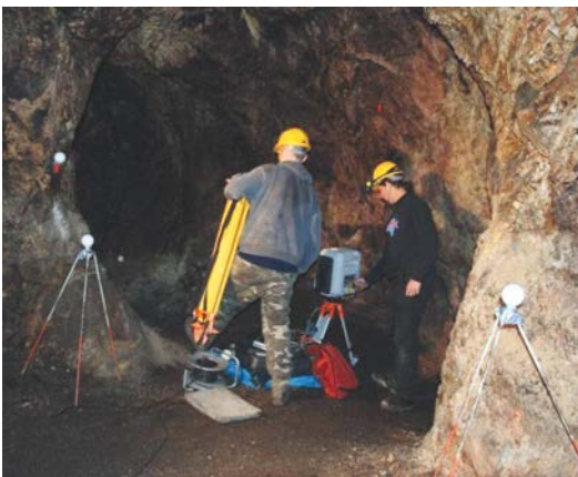
Fig. 1: Typical point cloud acquisition with a terrestrial laser scanner and artificial target spheres
