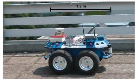
Fig. 1: Autonomous robot equipped with multi-sensor system for kinematic positioning and mobile mapping
