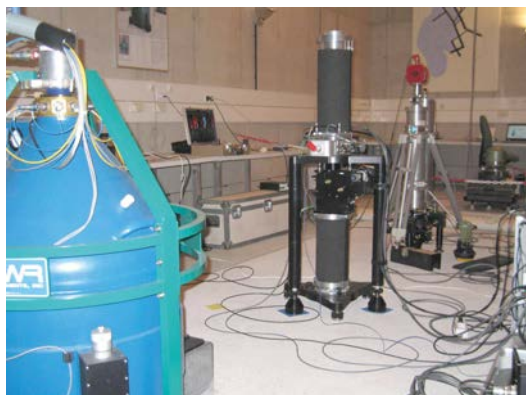
Fig. 5: Comparison of three types of gravimeters (GWR, FG5, JILAg) in the gravity laboratory at the Conrad Observatory Traflberg of ZAMG
