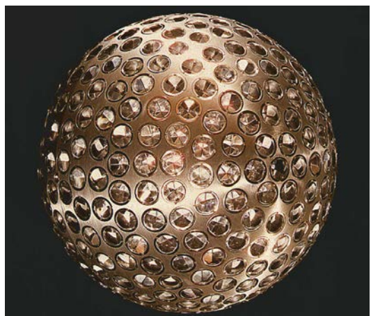
Fig. 1: Illustration of the LAGEOS-1 satellite. The surface of the passive satellite is covered by 426 laser retro-reflectors (image credit: NASA).
