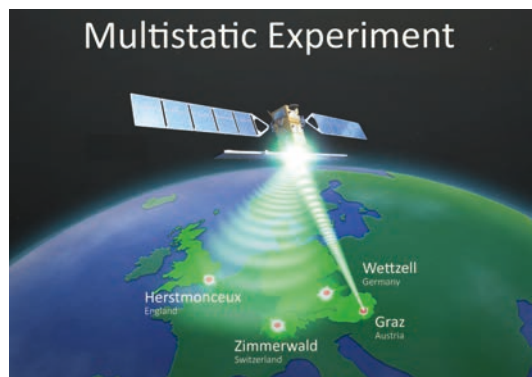
Fig. 4: Graz fired laser pulses to debris targets passing over Middle Europe; the photons - diffusely reflected from the debris targets - were detected at 4 SLR stations: Graz; Zimmerwald (600 km); Wetzell (400 km); Herstmonceux (1200 km); Graphics: Peter Ruzek/ AIUB
