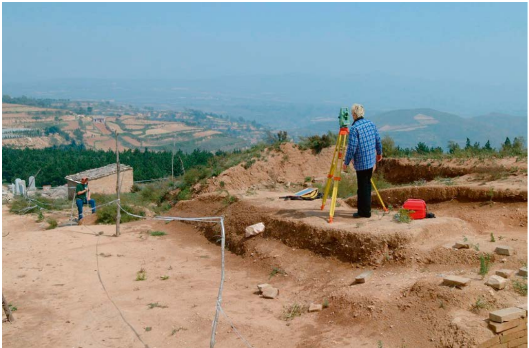
Fig. 1: Recording of archaeological findings using tachymetry
