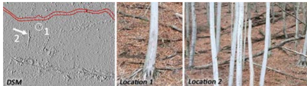
Fig. 4: DSM produced from full-waveform ALS point cloud cut of at 2 m height difference to DTM. Individual and fallen trees are clearly visible. The two images on the right were taken on-site and geo-referenced with GPS. [62]
